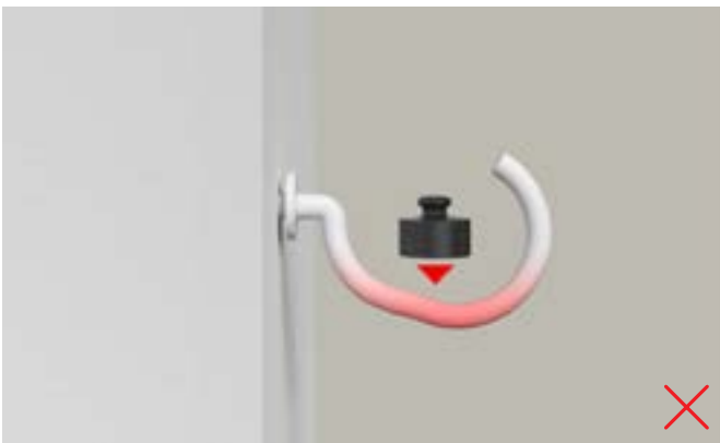
Steel hooks with a small material diameter deform more quickly and can no longer carry the full load.
