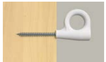
To achieve a smaller wall distance, you can use the hook without the shaft cone. To do this, simply break off the front part by hand.
